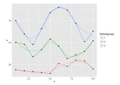
An X-spline is a line drawn relative to control points. For each control point, the line may pass through (interpolate) the control point or it may only approach (approximate) the control point; the behaviour is determined by a shape parameter for each control point.
